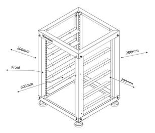
**Note:** There should be no obstacles within 600mm in front of the cabinet installation location and within 200mm on the other three sides.
