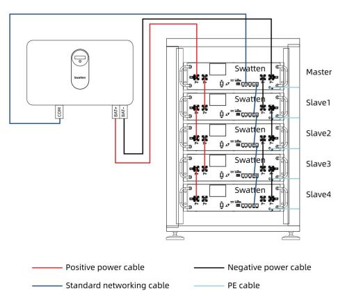
Figure 5.1 Battery Wiring Overview Diagram
