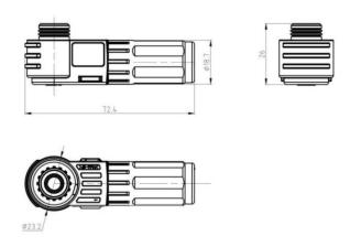
Figure 5.1 Battery Terminal Diagram
